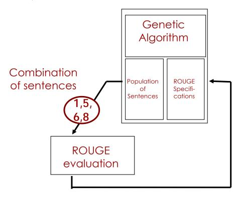
Figure 4.8 – Scheme of the proposed genetic algorithm.
